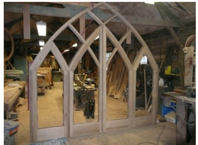
Interior doors for a chapel, under construction in Tim's workshop
